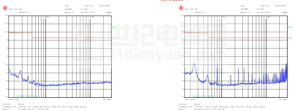
Figure: EMI scans per EN50121-3-2 for 43 -  $154V_{IN}$  to  $24V_{OUT}$  DC system
