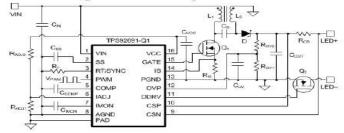
E.g. SEPIC from VIN from 7 – 16 V, VLED = 2 V for Red LED  Flexibility on sensing resistor position: either high-side or low-side
