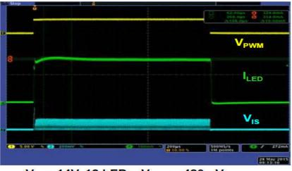
$V_{\text{IN}} = 14V, 18 \text{ LEDs}, V_{\text{IADJ}} = 420 \text{mV}, \\ R_{\text{CS}} = 0.1\Omega, f_{\text{PWM}} = 400 \text{Hz}$
