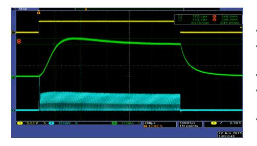
VIN = 14V, 18 LEDs, VIADJ = 420mV, RCS = 0.1Ω, fPWM = 400Hz
