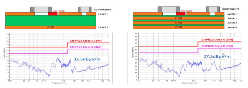
Two Layer (one GND layer) : 32.5 dBuV/m Multi layer GND shielding : 27.5 dBuV/m
