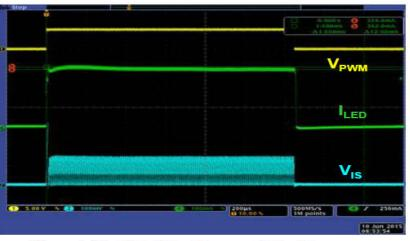
$V_{\rm IN} = 14V, 18 \text{ LEDs}, V_{\rm IADJ} = 420 \text{mV}, \\ R_{\rm cs} = 0.1\Omega, \, f_{\rm PWM} = 400 \text{Hz}$
