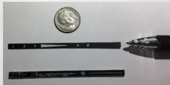
Sensors kit with high resolution slider, 3 mutual capacitance buttons, and 2 self capacitance buttons
